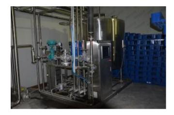
All the equipments and pipelines touching materials are made of stainless steel SUS304.
